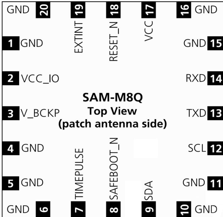
Figure 2: Pin assignment
